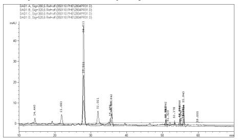
**Figure 1.** Example of phenolics separation: 1 – flavonols; 2 – phenolic acids; 3 – dihydrochalcones; 4 – quercetin glycosides
