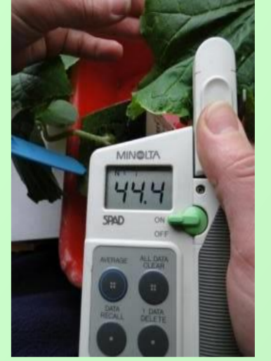
Leaf greenness evaluation using SPAD (Konica Minolta Japan)
